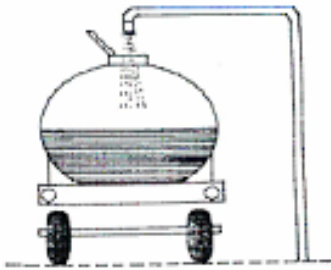
Figure 5-17: Air gap prevents back-siphoning
