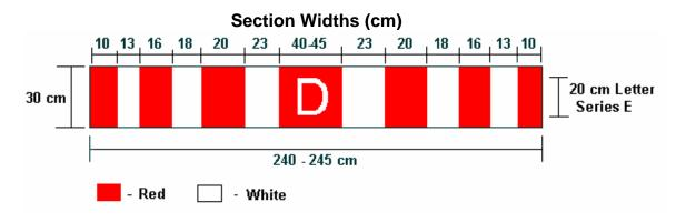
**Colour:** White – level II reflectance and stop sign red (# 712 3M) or equivalent **Material:** The sign panel must be fabricated of retroreflective material
