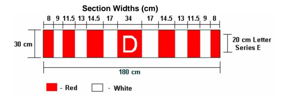
**Colour:** White – level II reflectance and stop sign red (# 712 3M) or equivalent **Material:** The sign panel must be fabricated of retroreflective material
