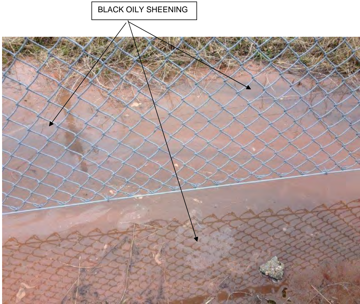
Photo 4-1 Petroleum sheening during air rotary drilling of 16MW20A and 16MW20B located on the IOL bulk plant property adjacent to 14 th St.
