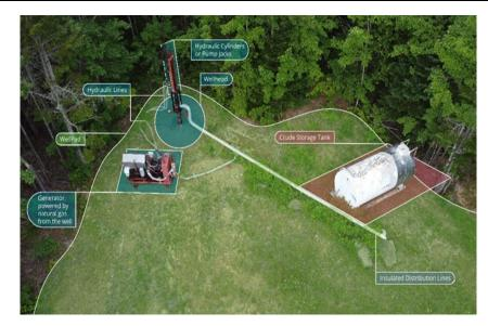
As in the photograph to the left, active crude oil wells have extraction and storage equipment that include a wellhead, pump jack, generator, transfer lines, and a storage tank. The number of actively producing crude wells varies at any given time and is dependent on crude market prices, production rates and transportation costs. As of March 2022, 12 crude oil wells were in production.
