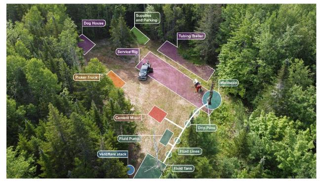
The supporting equipment will be positioned on the well pad to meet the required safety offsets from the well, and to efficiently conduct the decommissioning activities. All of the fluid transfer lines will be connected to the wellhead, fluid pump, and fluid holding tank or rig tank. Drip pans will be placed at each line connection to collect any released fluids.
