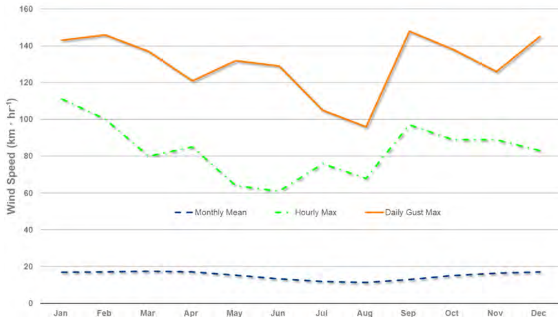
Figure 40. Compilation of wind speeds measured for the 30 year period between 1981 and 2010 at the Saint John Station A ( i.e. , Saint John airport).
