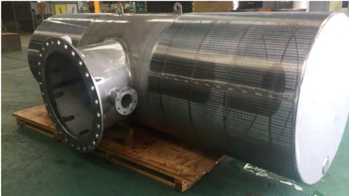
Figure 29. Photograph showing an example of a high-capacity, low-velocity intake screen.
