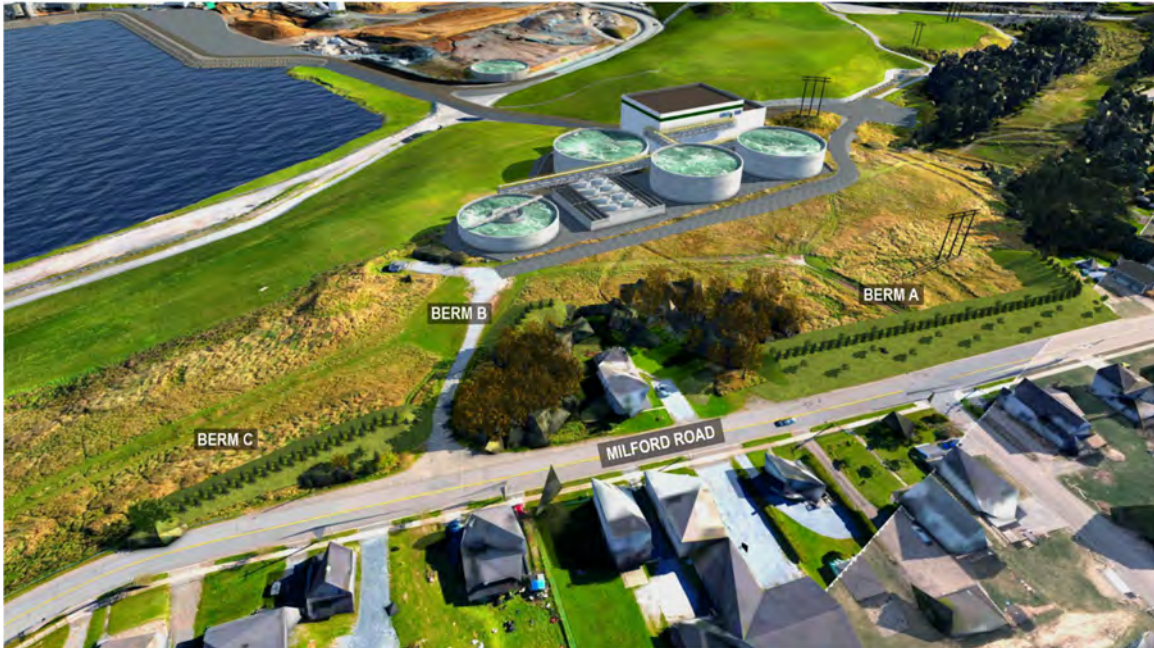
Figure 93. Conceptual image looking southeast towards the environmental treatment facility proposed for the Reversing Falls Mill in Saint John, New Brunswick. Note: the three sections of the berm are optional.
