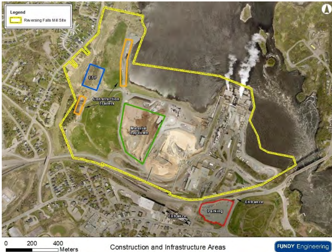
Figure 35. Aerial photograph of the Reversing Falls Mill in Saint John, New Brunswick showing the locations proposed for contractor project trailers, project parking areas, material laydown areas, and construction entrances for construction of the proposed environmental treatment facility and water use reduction project.
