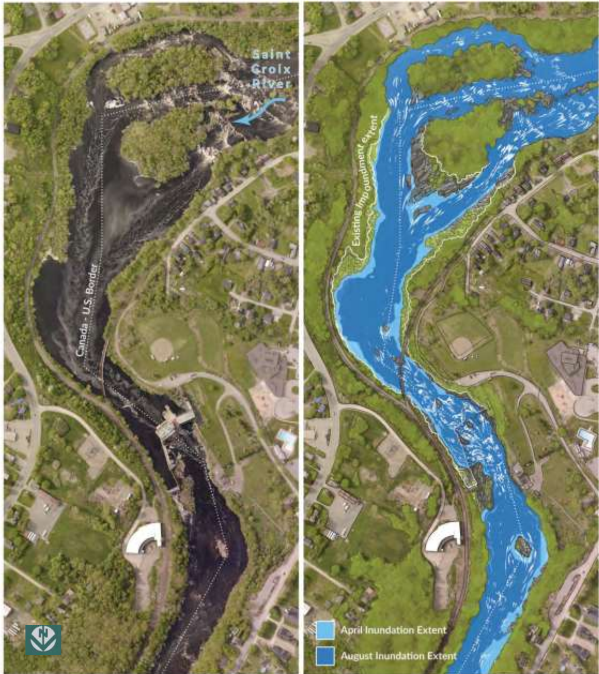
Figure 2.3.2: Conceptual Artists' Rendering Following the Completion of Bank-to-Bank Decommissioning and Removal – Plan View
