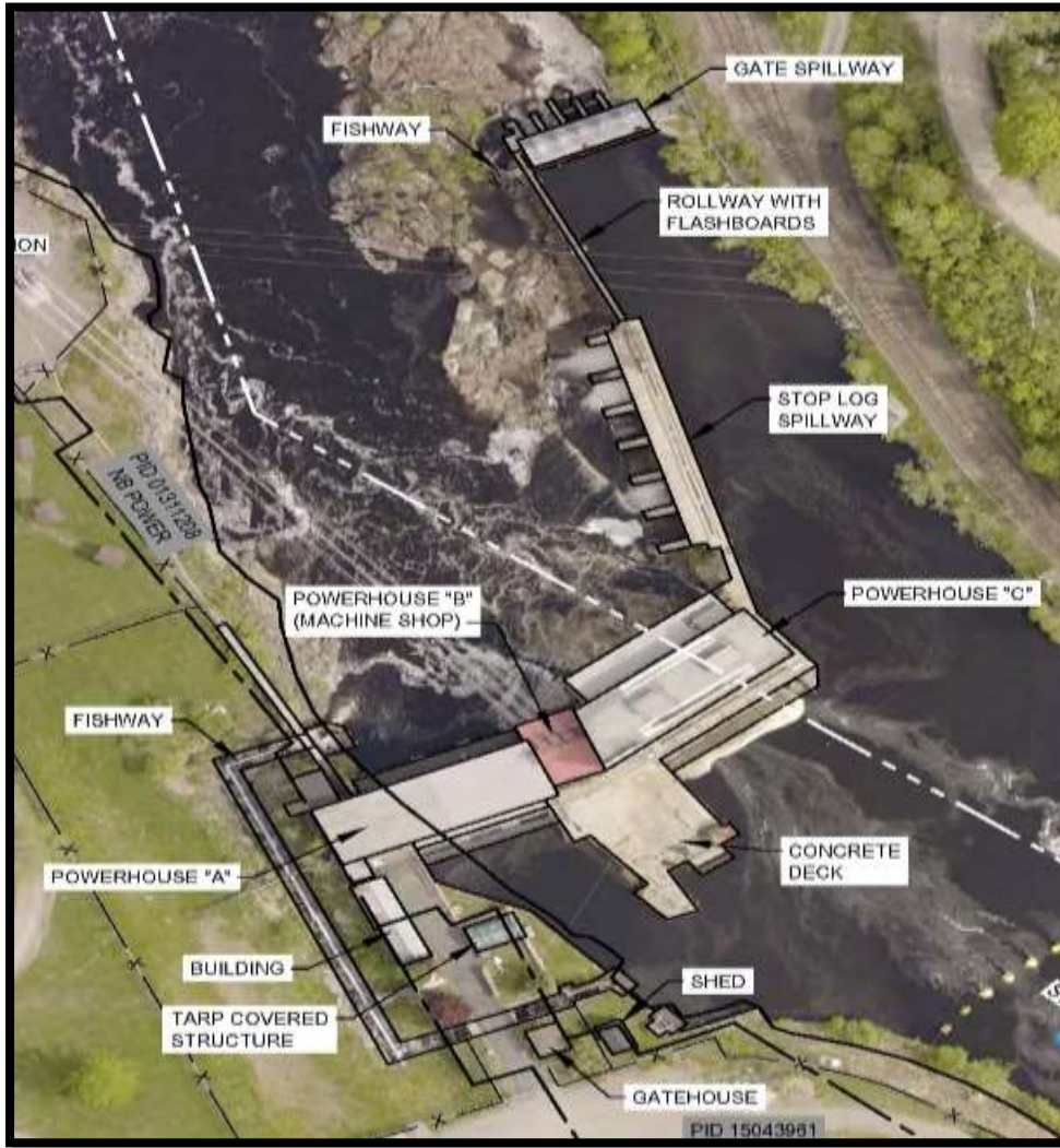
Figure 5.5.2: Key Features of the Milltown Dam (GHD and Inter-Fluve 2020)
