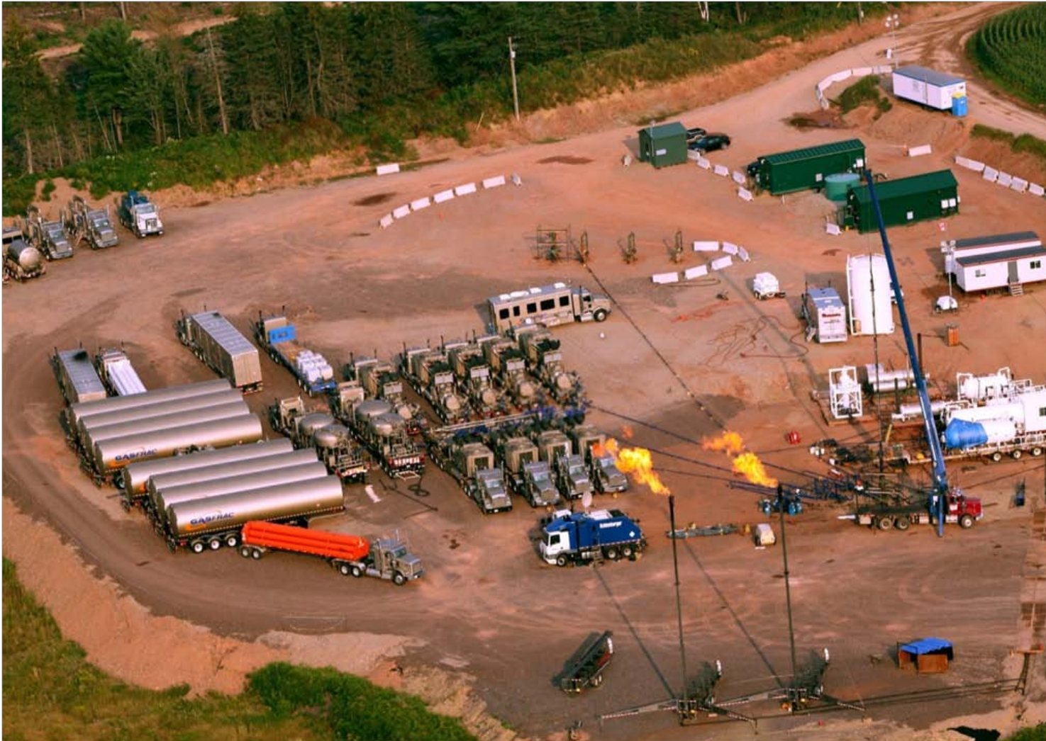
Figure 2.2 Typical Layout of Fracture Stimulation Equipment in NB
