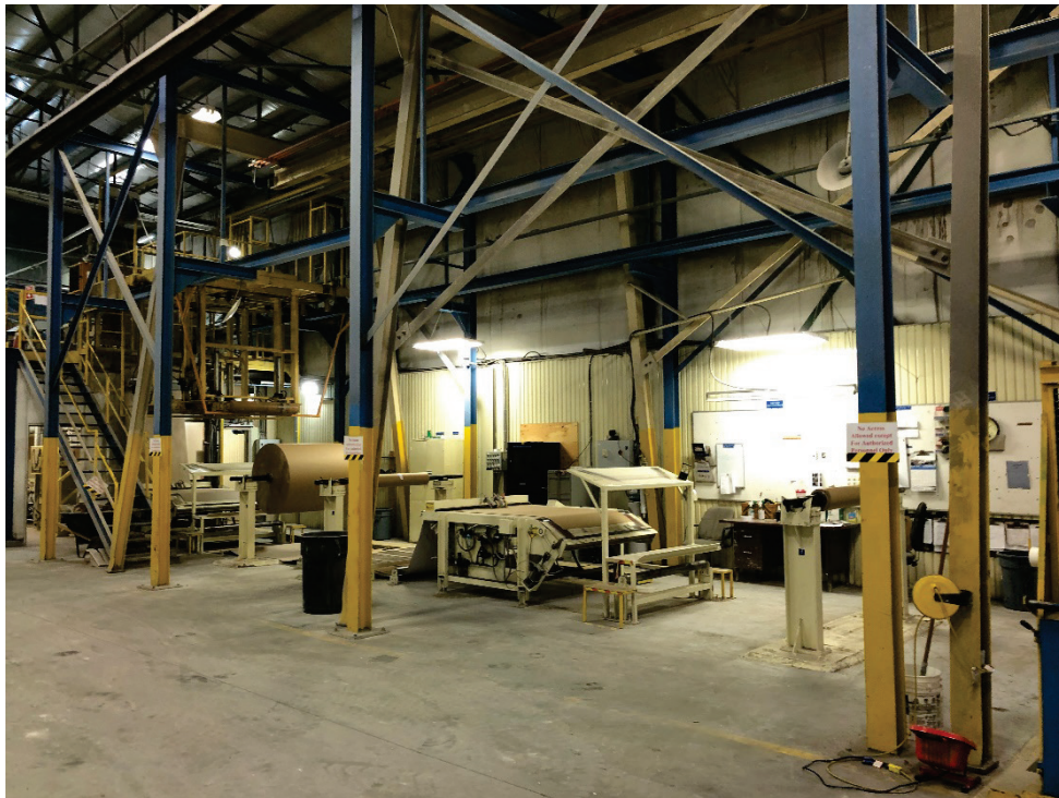
Photo 11 - Photo of unwind stand in paper staging area.
