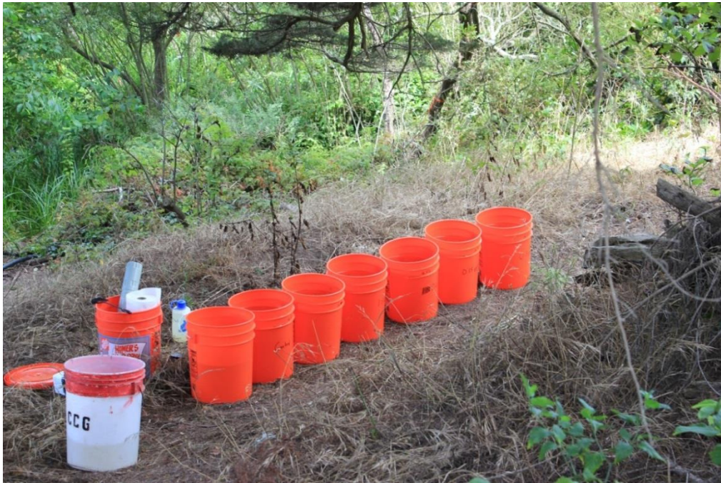
Figure 5.6. Field bioassay using serial dilutions of rotenone in plastic buckets to estimate site-specific toxicity to target species.
