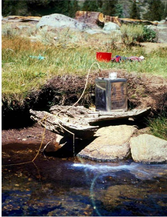
Figure 7. Drip station applying liquid rotenone to a stream (See SOP 11.1; Finlayson et al. 2018).
