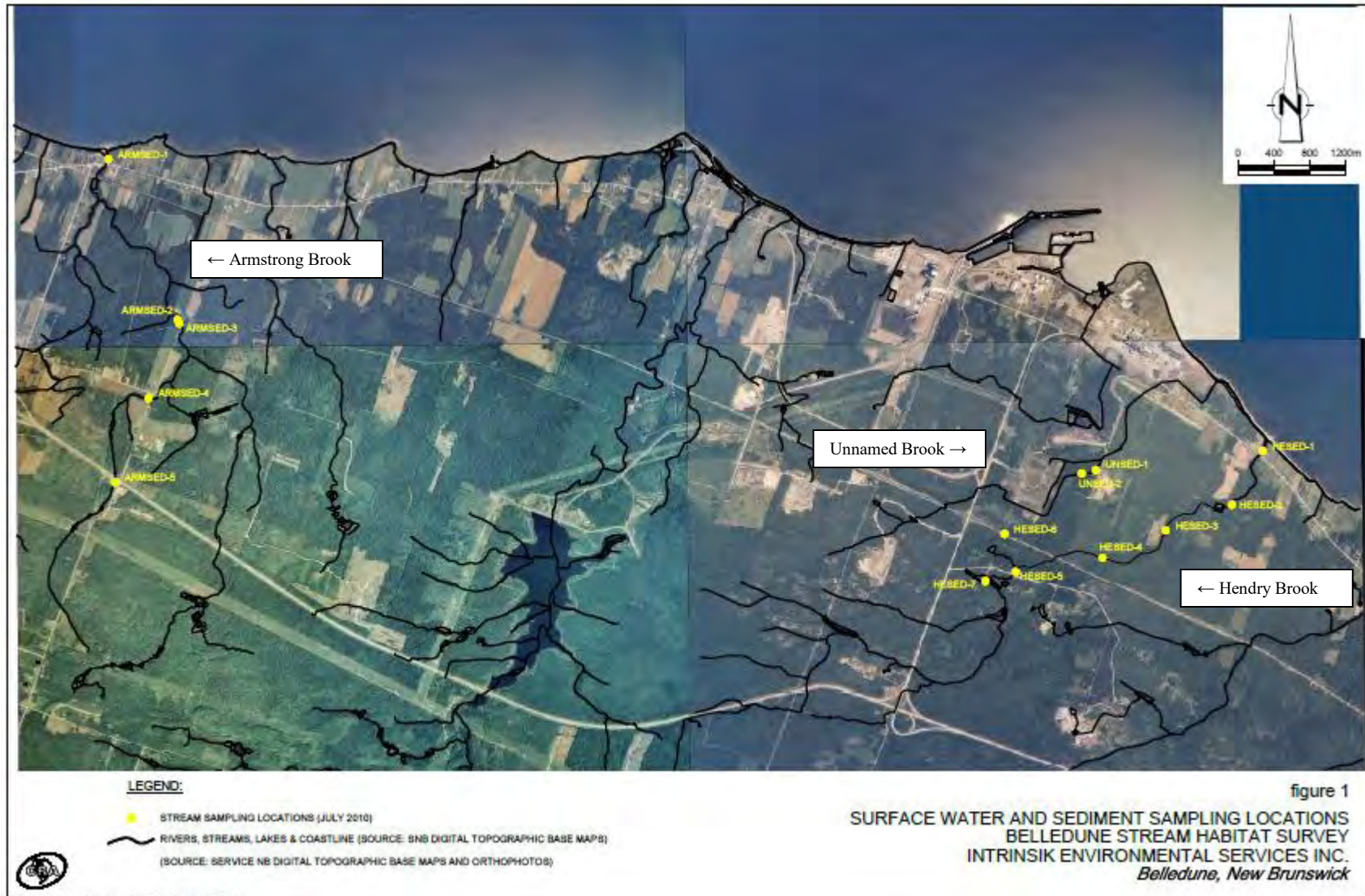
Figure 4-3 Location of Brook Surface Water and Sediment Sampling Locations
