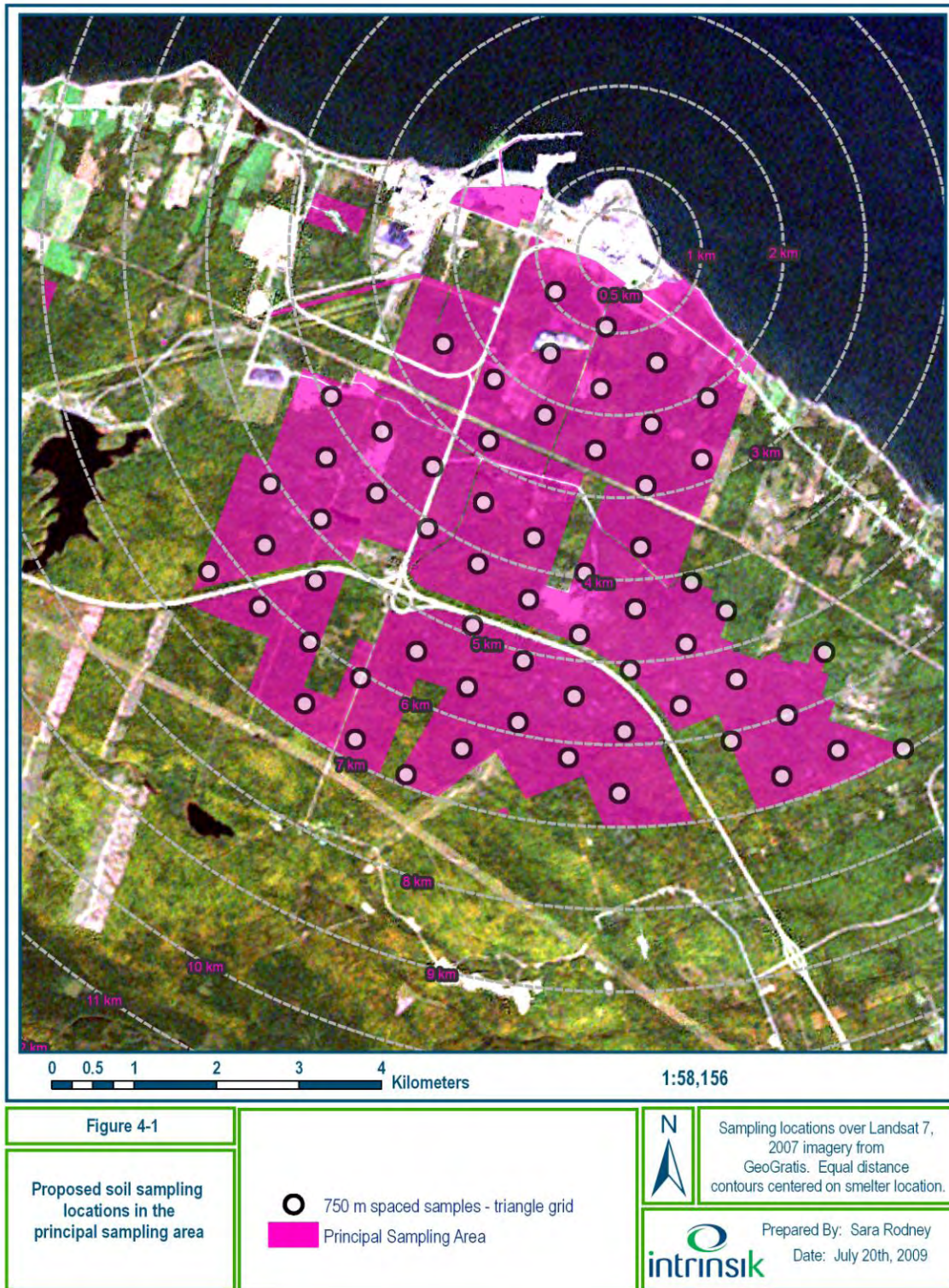
Figure 4-1 Principal sampling area and proposed soil sampling locations in the area surrounding the Xstrata Zinc Lead Smelter near Belledune, New Brunswick.
