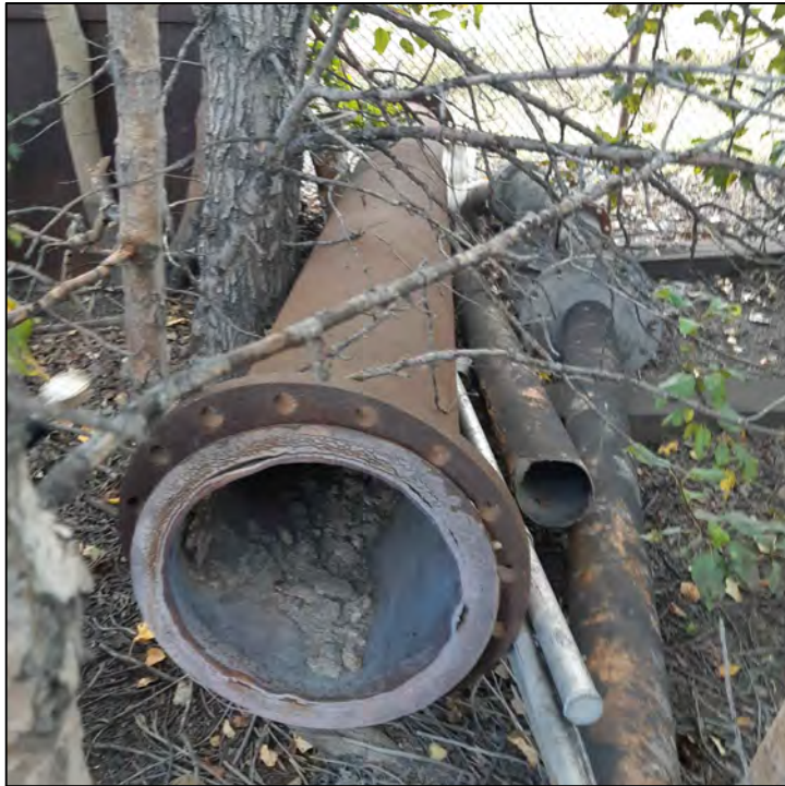
PHOTO 3 - GYPSUM PIPING IN SCRAP YARD
