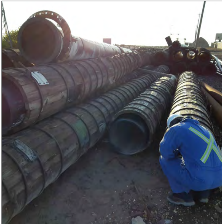
PHOTO 21 - GYPSUM LINE STOCKPILED ON THE NORTH SIDE OF THE SMELTER AREA. APPROXIMATELY 25 SECTIONS OF PIPING THAT ARE 30 FEET IN LENGTH
