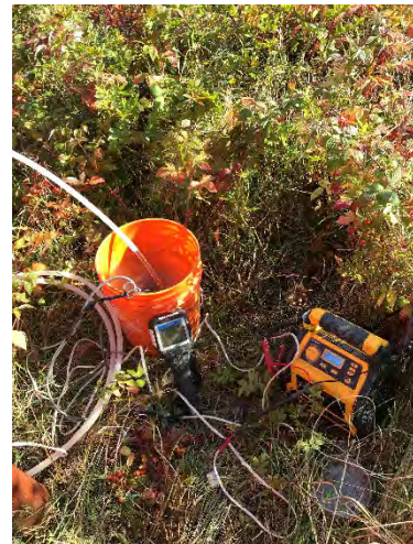
Photo #12: View of groundwater monitoring and purging equipment set up at existing monitor well 05GW-76.
