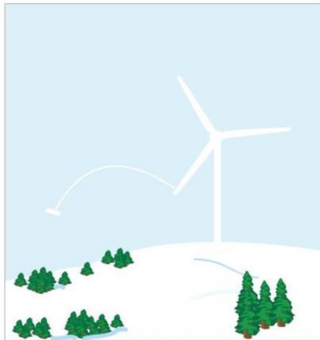
Figure 1: Schematic representation of Ice Throw
