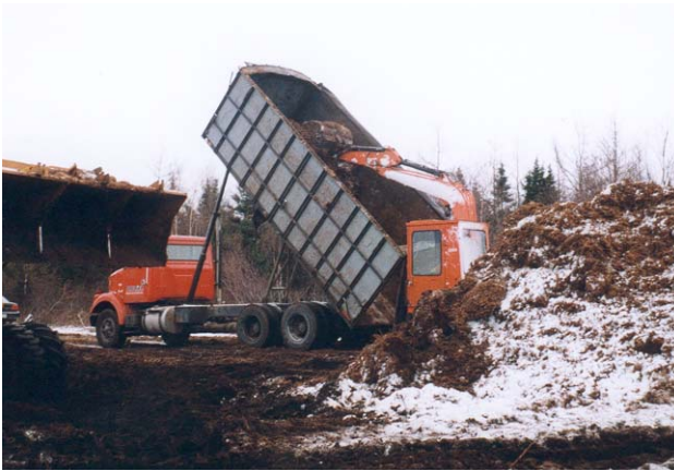
Figure 14. Photo showing the consequence of plant material freezing in trucks or trailers when temperature drops below 0 degree Celsius. (Photo : F. Quinty)
