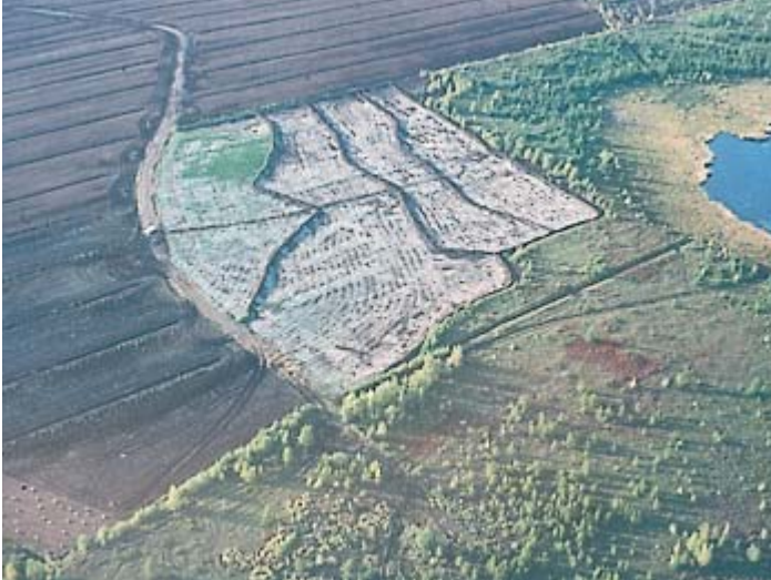
Figure 9. Aerial photo of Inkerman Ferry restoration site, New Brunswick. Across slope berms were built along contour lines after the site was surveyed. Restoration work took place in the fall of 1997 and the photo was taken in September 1998. (Photo: F. Quinty)
