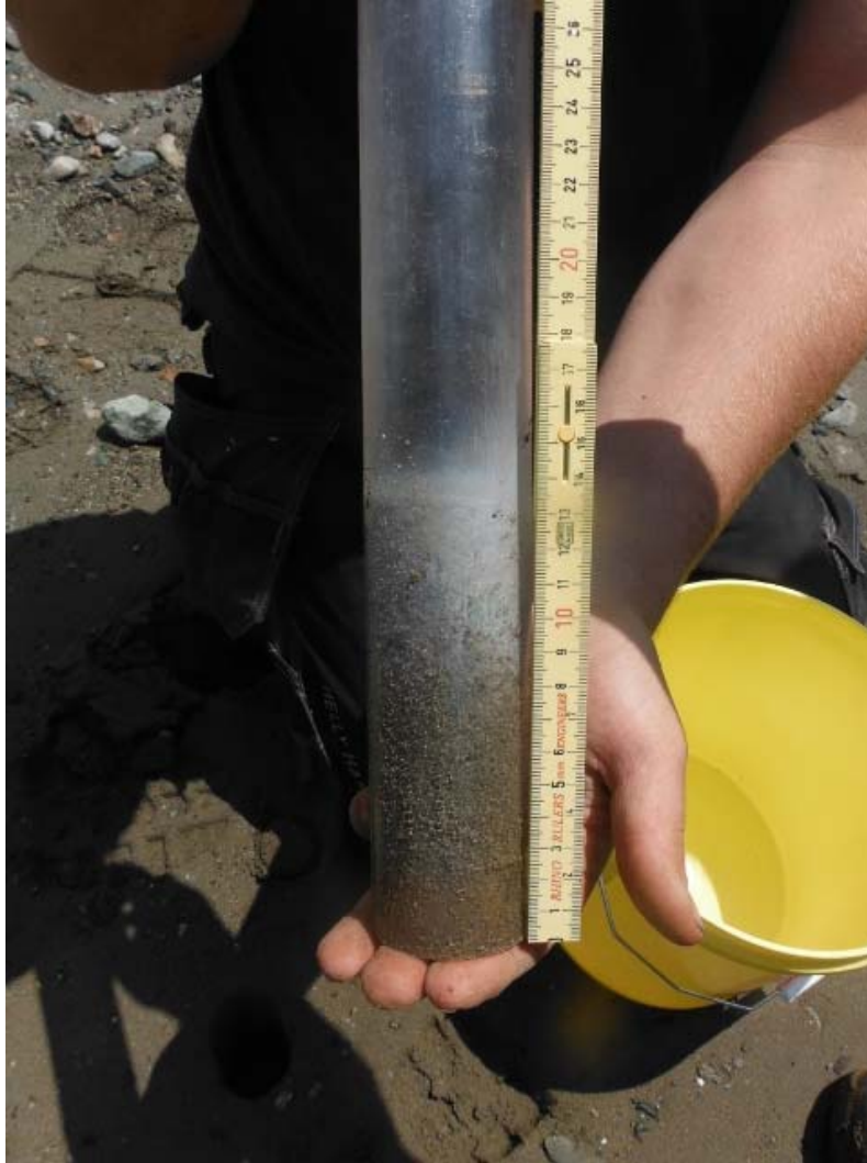
Typical depth of penetration of core tubes ~12 cm
