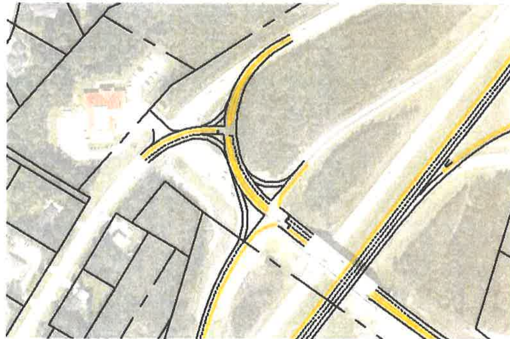
Figure 10: Concept Sketch of IC-4 (Realignment of Campbell Drive)
