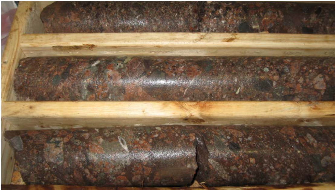
Photo 2 – Conglomerate Bedrock Core (50mm dia) – into bedrock 2 metres
