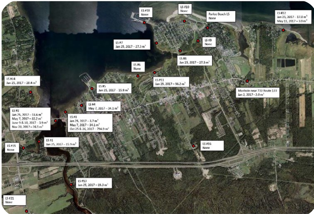
Figure 4.3k - GSSC Lift Station Overflows - 2017
