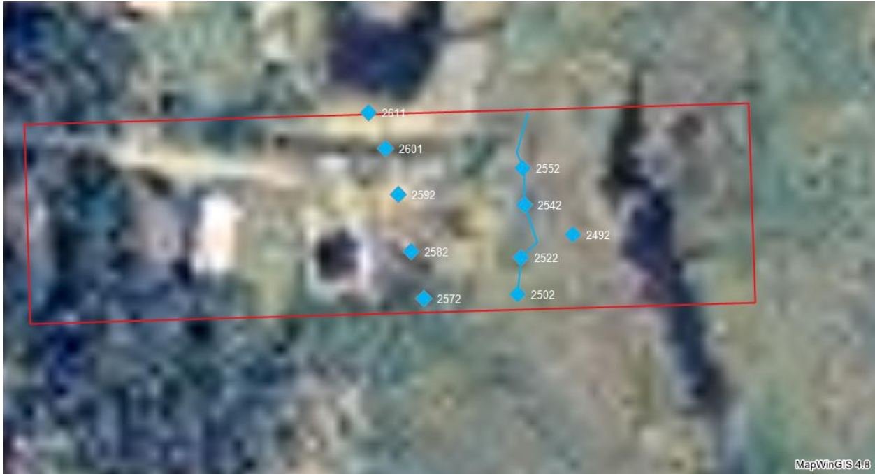
Figure 2. Sample Wetland Delineation Schematic. The red line is the property boundary. The blue line is the field-delineated wetland boundary (wetland to right, upland to left) with GPS points taken along the line. The single point east of the wetland boundary is the location at which a wetland data sheet was completed. The second series of points depicts the upper boundary of dunes or coastal features which are not wetlands but are considered habitat of conservation concern.
